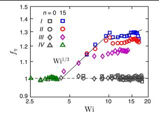
FIG. 4. Viscous friction factor  $f_{\eta}$  as a function of Wi for n = 0 and 15 with four cases and types of polymeric fluids. Case I: 300 ppm PAA 90% glycerol, 0–50 W, II: 50–290 W, III: 250 ppm PAA 90% glycerol, 0–290 W, IV: 100 ppm PAA 93% glycerol, 0–290 W.
