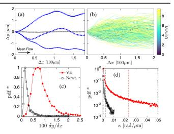
FIG. 5. (a) Particle trajectories in the streamwise (x) and spanwise (y) direction; blue lines represent the n = 15 viscoelastic case at Wi = 18 and the gray line is Newtonian at identical conditions. (b) Collection of trajectories colored by speed. Distributions of (c) cumulative transverse to streamwise displacements and (d) trajectory curvatures, where the dashed line represents population mean.
