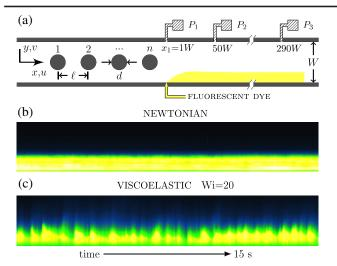
FIG. 1. (a) Schematic of the microchannel, showing location of pressure sensors and the dye injection scheme. [(b) and (c)] Spacetime dye patterns for n = 15 and x = 200 W in the parallel shear region, (c) viscoelastic fluid at Wi = 20, and (b) the Newtonian case at identical flow rate.
