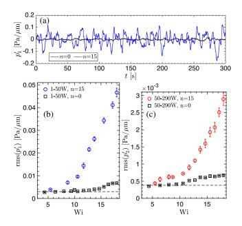
FIG. 3. (a) Pressure gradient signal  $p'_1(t)$  for the n = 15 case, compared with the unperturbed n = 0 case, Wi = 18. [(b) and (c)] Root-mean-square (rms) fluctuations versus Wi for n = 0 and 15, (b)  $p'_1$ , and (c)  $p'_2$ . The dashed line is the average level for Newtonian fluid, experimentally found to be constant for increasing Q.
