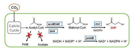
**Fig. 10.5** Scheme of biosynthetic pathway of 3HP from  $CO_2$  in engineered *Synechocystis* sp. PCC 6803 [32]. The malonyl-CoA reductase was encoded by gene *mcr*. Acetyl-CoA carboxylase was encoded by genes *accB*, *accC*, *accA*, and *accD*. Biotinilase was encoded by gene *birA*. The NAD(P) transhydrogenase was encoded by gene *pntA* and *pntB*
